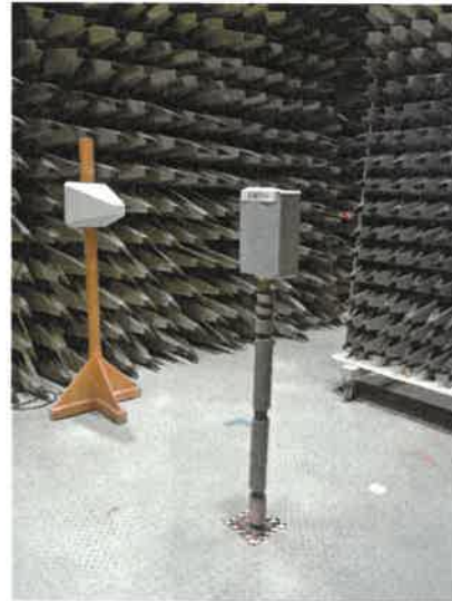
Figure 11: Shielding effectiveness measurement of the back side in the frequency range 1 GHz – 4 GHz
