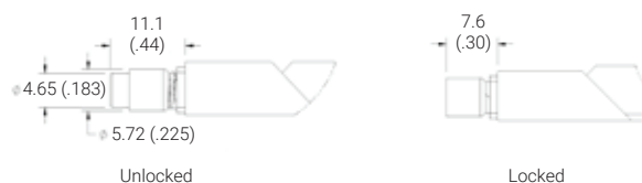
Detail "V" Provides visual lock indication.
