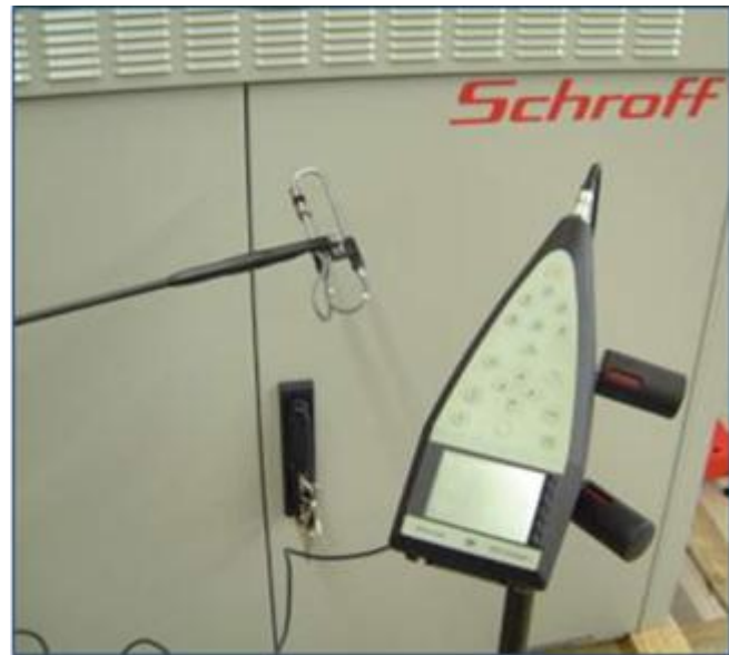
Figure 6 Test equipment acoustic noise measurements
