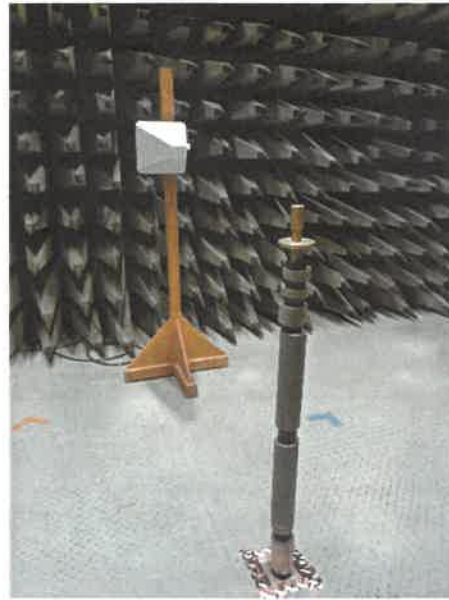
Figure 7: Dynamic range measurement
