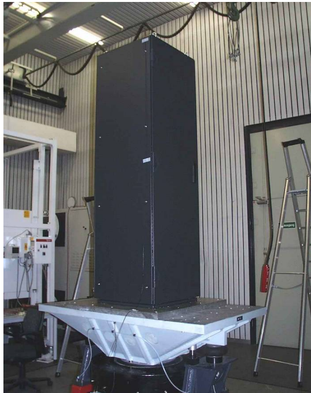
Pic. 2 Mounting of EUT Z-Axis (Vibration Response Investigation)e
