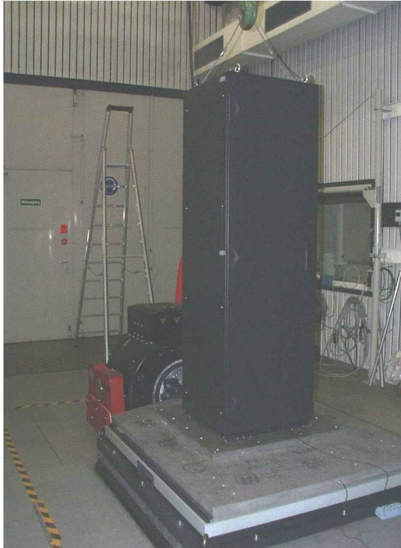
Pic. 3 Mounting of EUT X-Axis (Vibration Response Investigation)
