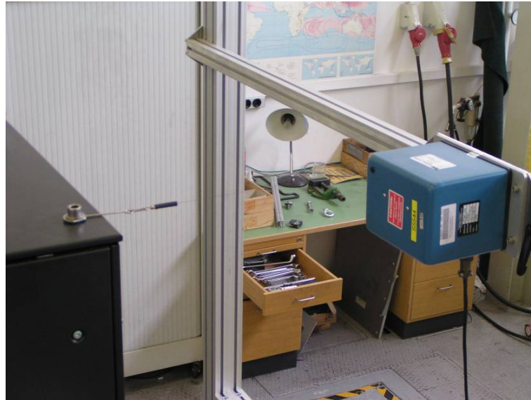
Pic. 6 Measuring equipment LVTD for displacement
