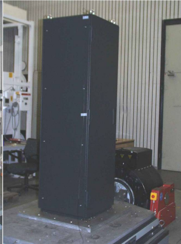
Pic. 4 Mounting of EUT X-Axis (Vibration Response Investigation) Example
