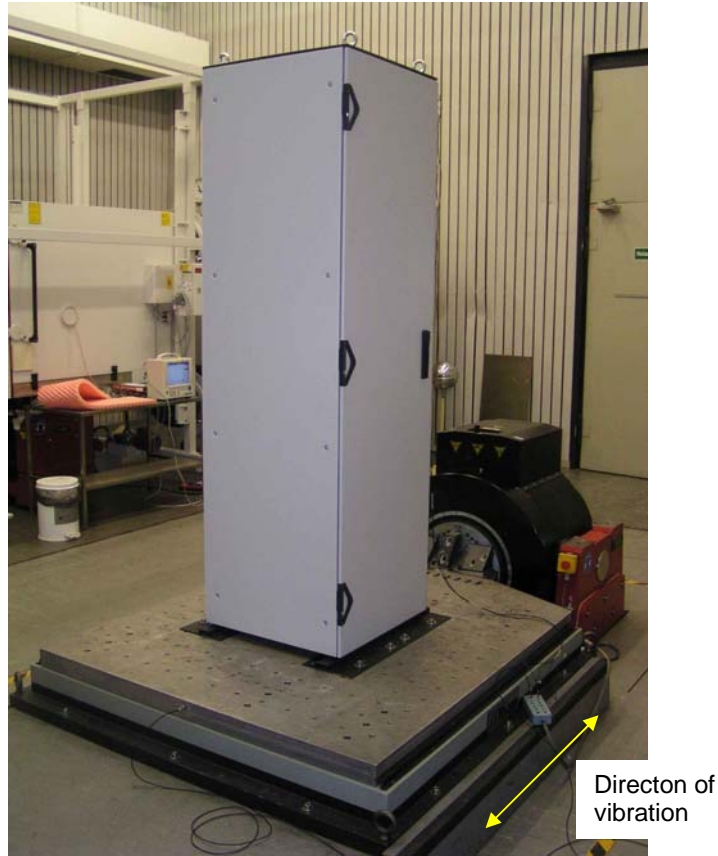
Photo 1: EUT mounted at vibration table. Axis of vibration X – longitudinal (side - side)
