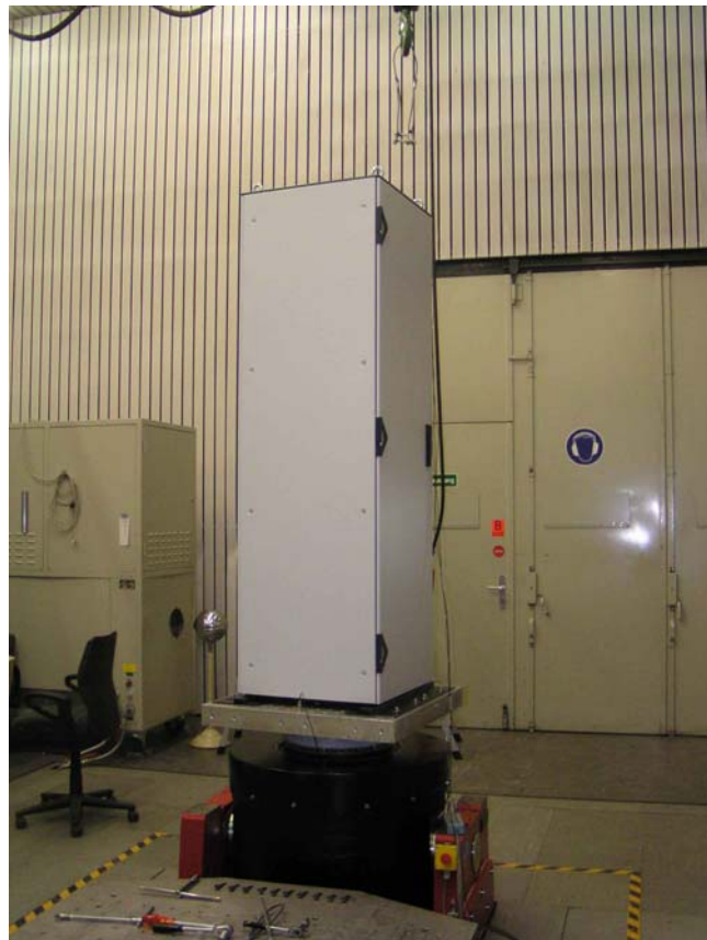
Photo 3: EUT mounted at vibration table. Axis of vibration Z (vertical)
