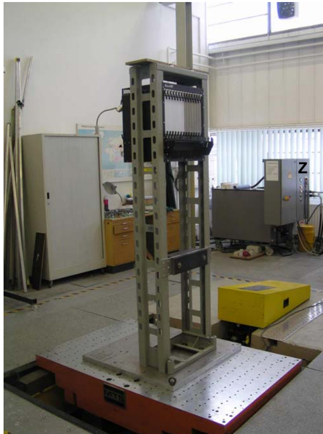
Photo 4: Mounting of EUT for Z-axis test (14 dummy board front and 14 dummy boards rear)
