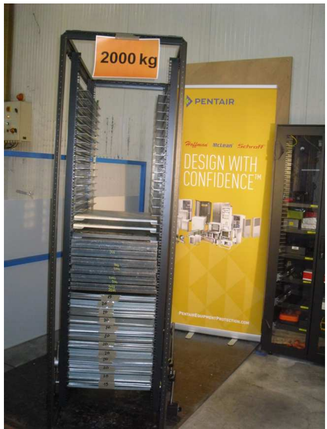
Picture 2 Frame loaded with 2000 kg
