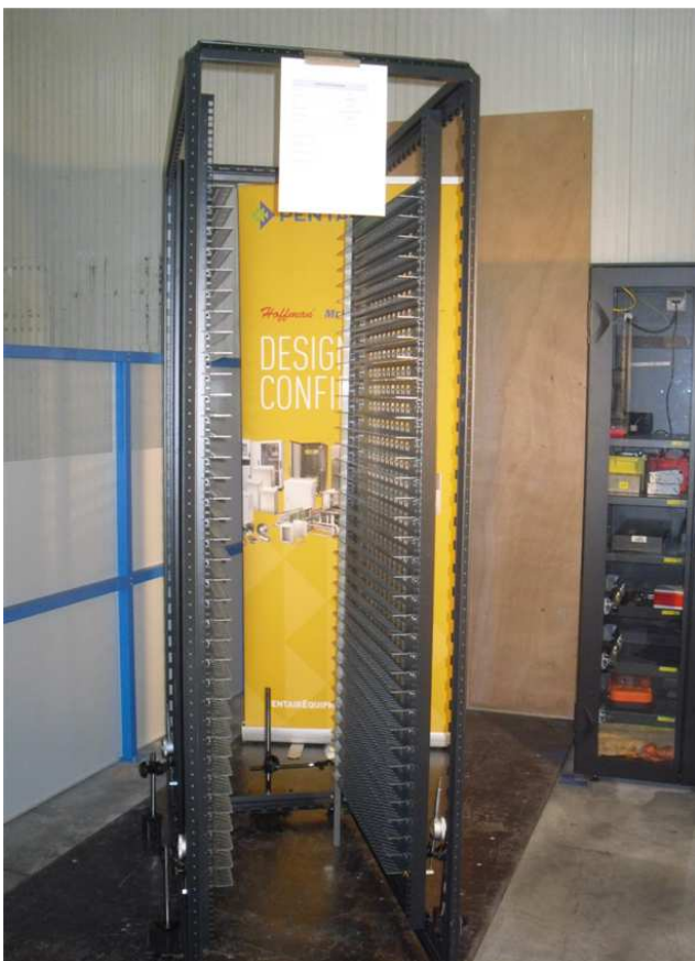
Picture 1 Frame with the 36 pairs of slide rails
