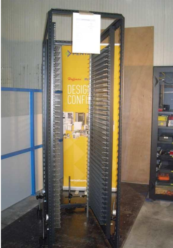
Picture 1 Frame with the 36 pairs of slide rails
