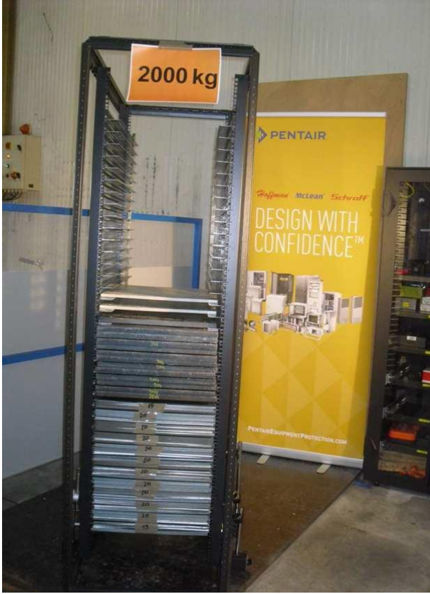
Picture 2 Frame loaded with 2000 kg
