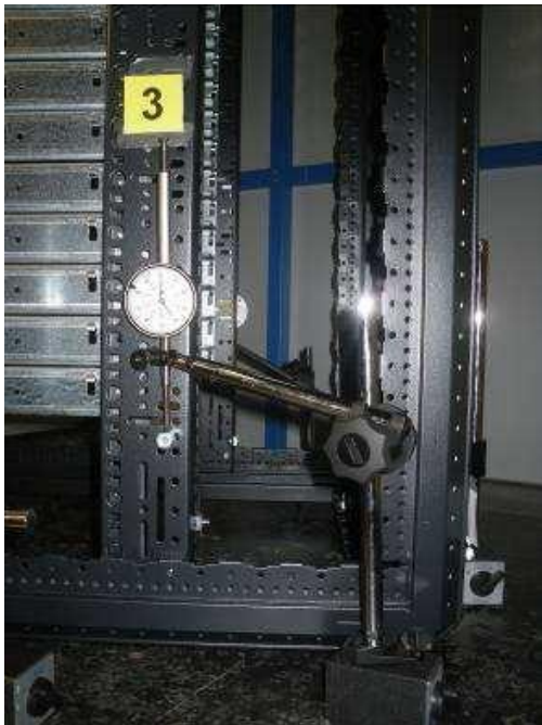
Picture 3 Dial indicators to measure panel mount displacement
