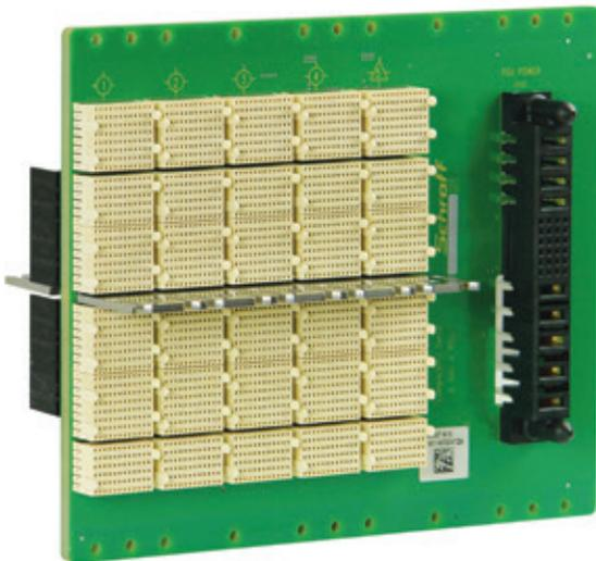
The SCHROFF backplane family offers a enormous number of different combinations. The connector for the pluggable power supply can be either integrated on the backplane, or linked with a power adapter board which connects the 12 V and GND between SCHROFF CompactPCI Serial power backplanes and backplanes. With the available space of the 19" chassis the user could add additional power supplies for power redundancy or even realize several independent CPCI Serial systems in one chassis.
