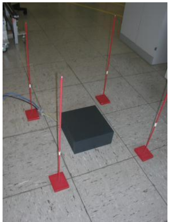
Figure 22 Measurement setup Acoustic Noise-2
