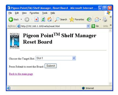
After the user chooses the target slot number and clicks the "Submit" button, the request is executed and the results page is shown, similar to the one below. This command is essentially equal to the CLI command boardreset.
