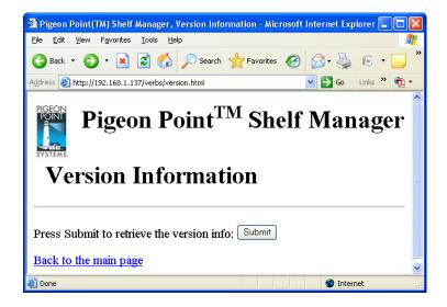
After the user clicks the "Submit" button, the request is executed and a results page similar to the following one is shown. The output is essentially equal to the output produced by the CLI command version.
