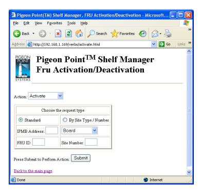
After the user fills in all fields and clicks the "Submit" button, the request is executed and the results page is produced, similar to the one below. This command is essentially equal to one of the CLI commands activate, deactivate or setlocked, depending on the action chosen.
