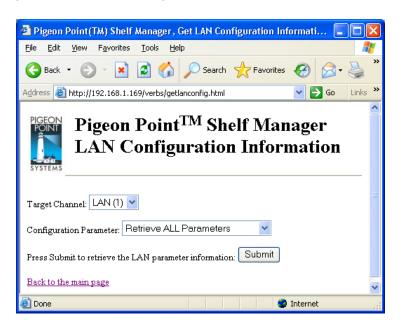
After the user fills in the request information and clicks the "Submit" button, the request is executed and the results page is generated, similar to the one below. The output produced by this command is essentially the same as the output produced by the CLI command getlanconfig.
