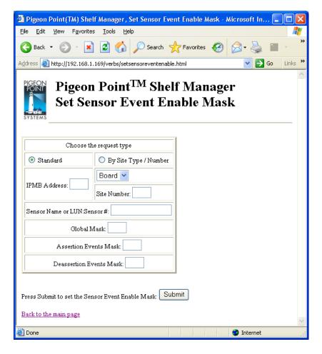
For example, if the request specifies sensor 3 without explicit LUN qualification, and the target controller exposes sensor 3 on LUN 1 and another sensor 3 on LUN 3, the action is applied to the sensor 3 on LUN 1.
