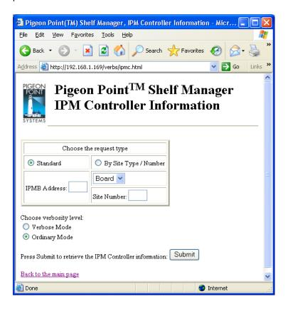
After the user fills in the desired fields and clicks the "Submit" button, the request is executed and a results page is shown, similar to the one below. The output is essentially equal to the output produced by the CLI command ipmc.
