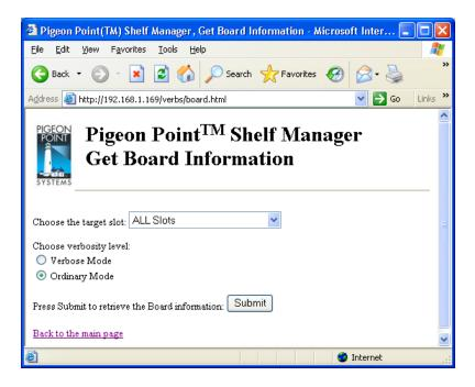
After the user fills in all fields and clicks the "Submit" button, the request is executed and the results page is shown, similar to the one below. The output is essentially equal to the output produced by the CLI command board.
