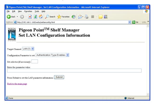
After the user specifies all necessary information and clicks the "Submit" button, the request is executed and the results page is shown, similar to the one below. This command is essentially equal to the CLI command setlanconfig.
