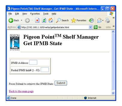
After the user fills in the request information and clicks the "Submit" button, the request is executed and the results page is generated, similar to the one below. The output produced by this command is essentially the same as the output produced by the CLI command getipmbstate.
