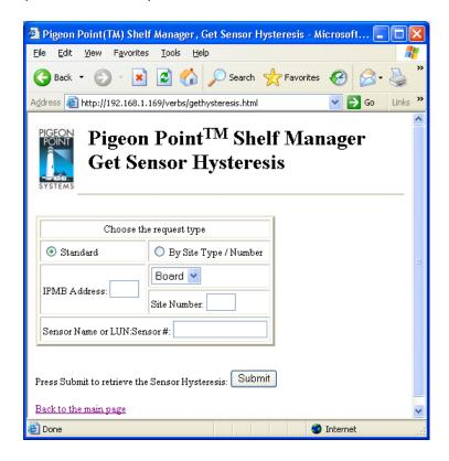
After the user fills in the desired fields and clicks the "Submit" button, the request is executed and the result page is shown, similar to the one below. The output is essentially equal to the output produced by the CLI command gethysteresis.
