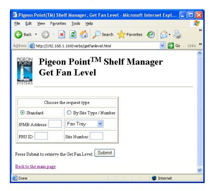
After the user fills in the desired fields and clicks the "Submit" button, the request is executed and the results page is shown, similar to the one below. The output is essentially equal to the output produced by the CLI command getfanlevel.
