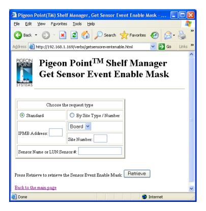
After the user fills in the request information and clicks the "Submit" button, the request is executed and the results page is generated, similar to the one below. The output produced by this command is essentially the same as the output produced by the CLI command getsensoreventenable.
