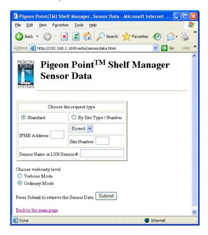
In the field "Sensor Name or LUN:Sensor #", the user can identify the target sensor by specifying the sensor name or specifying the sensor LUN and sensor number.
