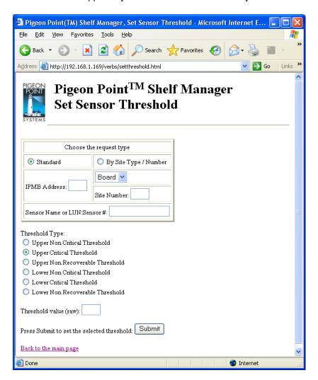
In the field "Sensor Name or LUN:Sensor #", the user can identify the target sensor by specifying the sensor name or specifying the sensor LUN and sensor number. In the last case, the LUN is optional; if specified, it is separated from the sensor number with a colon. Valid values for the LUN are 0, 1 and 3. (LUN 2 is reserved.)
