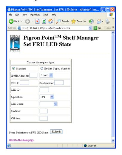
The optional parameter "LED Color" specifies a color, via a symbolic name. If the parameter is not specified, the default LED color is used. The possible values of "LED Color" are below:
