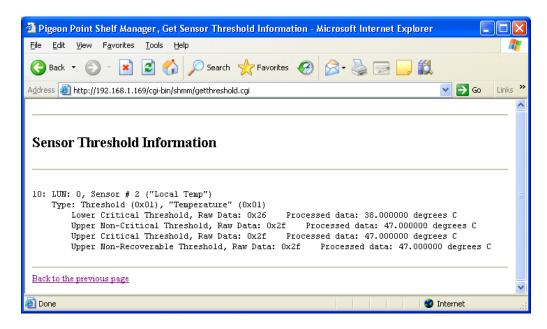
In the field "Sensor Name or LUN:Sensor #", the user can identify the target sensor by specifying the sensor name or specifying the sensor LUN and sensor number. In the last case, the LUN is optional; if specified, it is separated from the sensor number with a colon. If the user specifies only the sensor number, information is returned about known sensors with the specified sensor number on all LUNs. Valid values for the LUN are 0, 1 and 3. (LUN 2 is reserved.)
