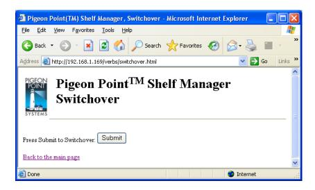
After the user clicks the "Submit" button, the request is executed and the following results page is shown. The output is essentially equal to the output produced by the CLI command switchover. Alternatively, the browser may report on an error because the Shelf Manager shuts down before the boa demon produces the results page.
