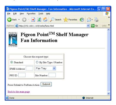
After the user fills in desired fields and clicks the "Submit" button, the request is executed and the results page is shown, similar to the one below. The output is essentially equal to the output produced by the CLI command fans.
