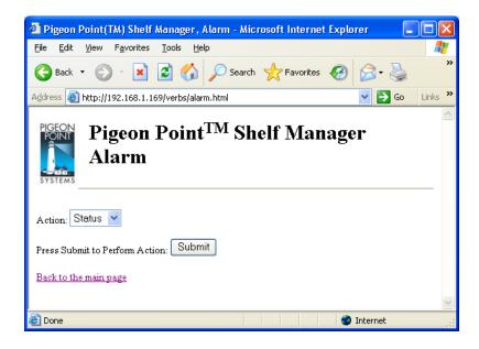
After the user selects one of the actions specified and clicks the "Submit" button, the request is executed and the results page is shown, similar to the one below. The output is essentially equal to the output produced by the CLI command alarm with a corresponding parameter.
