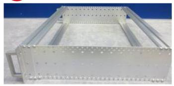
Customer needs 128HP wide subrack. The PCB weight was more than 200gr per PCB and the length was 280mm. To avoid a bending / deflection of the horizontal rail on the front side, a stiffen version of such a rail was requested.
