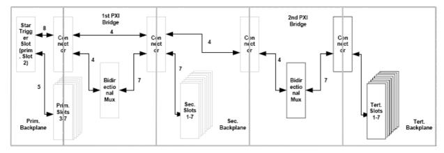
The structure of the multiplexers supports connections between any of the secondary or tertiary Star Trigger lines with one of the four primary Star Trigger lines. The following table gives an overview of the wiring of the Star Trigger lines.
