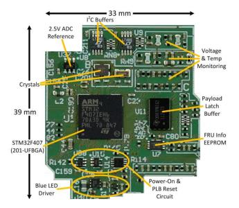
The photo in the left column shows the core of a BMR-STM32-ATCA IPMC. The active components are:
