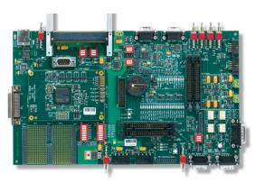
Supported SmartFusion intelligent mixed-signal FPGAs include the A2F200 and A2F500, with CS288, FG256 and FG484 packages. Please refer to Microsemi documentation for details of the differences in capabilities among these devices and see the separate *Pigeon Point BMR-A2F-VPX Product Brief* for more details on the reference design.
