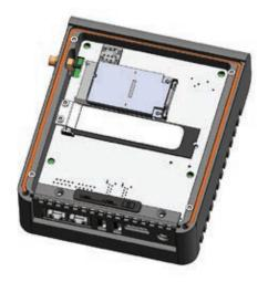
A round IP gasket is inserted into the gnotch in the case to seal the case parts to each other.
