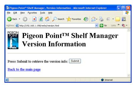
After the user clicks the "Submit" button, the request is executed and a results page similar to the following one is shown. The output is essentially equal to the output produced by the CLI command version.
