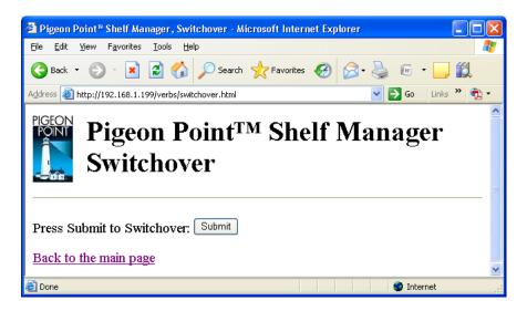
After the user clicks the "Submit" button, the request is executed and the following results page is shown. The output is essentially equal to the output produced by the CLI command switchover. Alternatively, the browser may report on an error because the Shelf Manager shuts down before the boa demon produces the results page.
