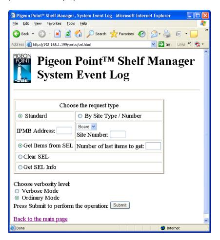
After the user chooses the upper radio option and fills in desired fields and clicks the "Submit" button, the request is executed and the results page is shown, similar to the one below. The output is essentially equal to the output produced by the CLI command sel.
