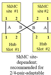
The shelf manager Ethernet ports in a Schroff shelf are wired according to the ATCA site-dependent diagram at the left. If only a single switch blade is installed in slot #1, and a shelf manager switchover occurs, shelf manager #2 will not have network connectivity because its port #1 is wired to Hub slot #2 and port #2 is not used in the default configuration.
