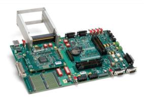
Supported SmartFusion intelligent mixed-signal FPGAs include the A2F200 and A2F500 with the CS288, FG256 and FG484 packages. Please refer to Microsemi documentation for details of the differences in capabilities among these devices and see the separate *Pigeon Point BMR-A2F-AMCc Product Brief* for more details.
