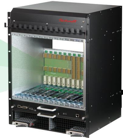
100G Backplane assembled into SCHROFF NextGen ATCA Chassis
