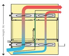
The air intake is at the front bottom side of the chassis, the air exhaust is the rear upper side. Air baffles separate the air flow for the front card section and the rear card section in order to maximize cooling capability.
